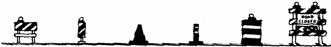
Barricade Pane Cone Tube Drum Barricade
