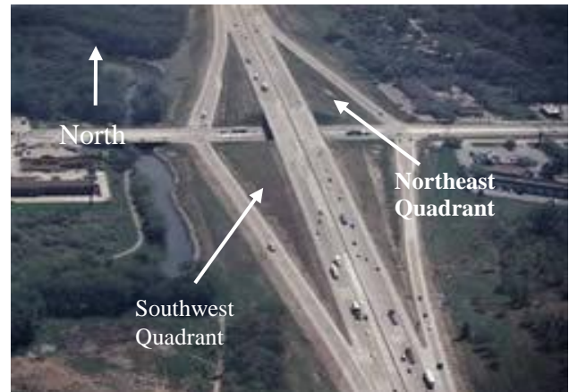
“DIAMOND INTERCHANGE” If the general north direction of the highway is towards the top of the page then the top left portion of the interchange would be the northwest quadrant; the top right would be the northeast quadrant; the bottom left would be the southwest quadrant and the bottom right would be the southeast quadrant.”
