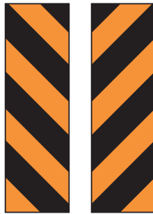
Hazard to left Hazard to right
