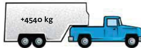
Truck pulling a trailer with a GVW of more than 4540 kg (Class 3)
