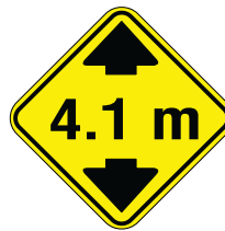
Low structure clearance 4.1 m
